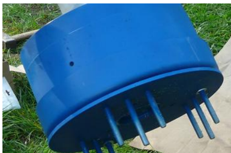
Threaded bolts on generator (for rotorblades Airfoil E387)
